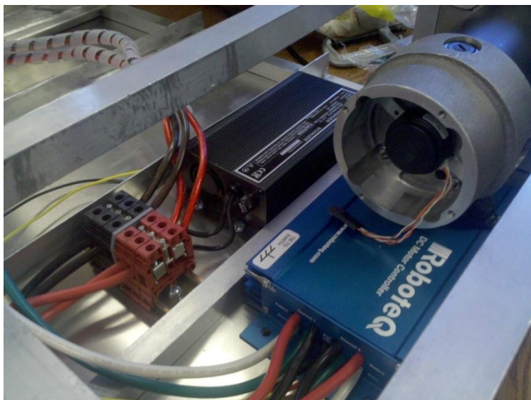
Figure 3: Distribution hub, on-board charger, motor controller, and motor with encoder
