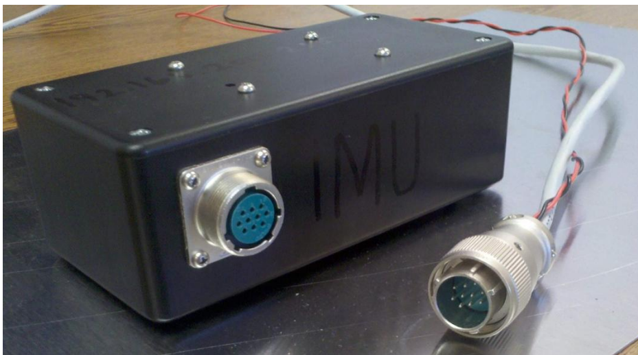
Figure 5: Sensor node with example Ethernet/Power cable
